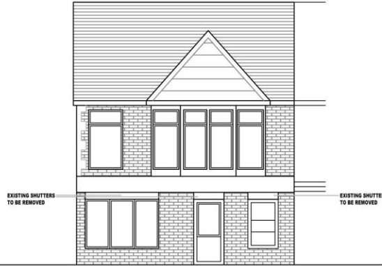
EXISTING FRONT ELEVATION
